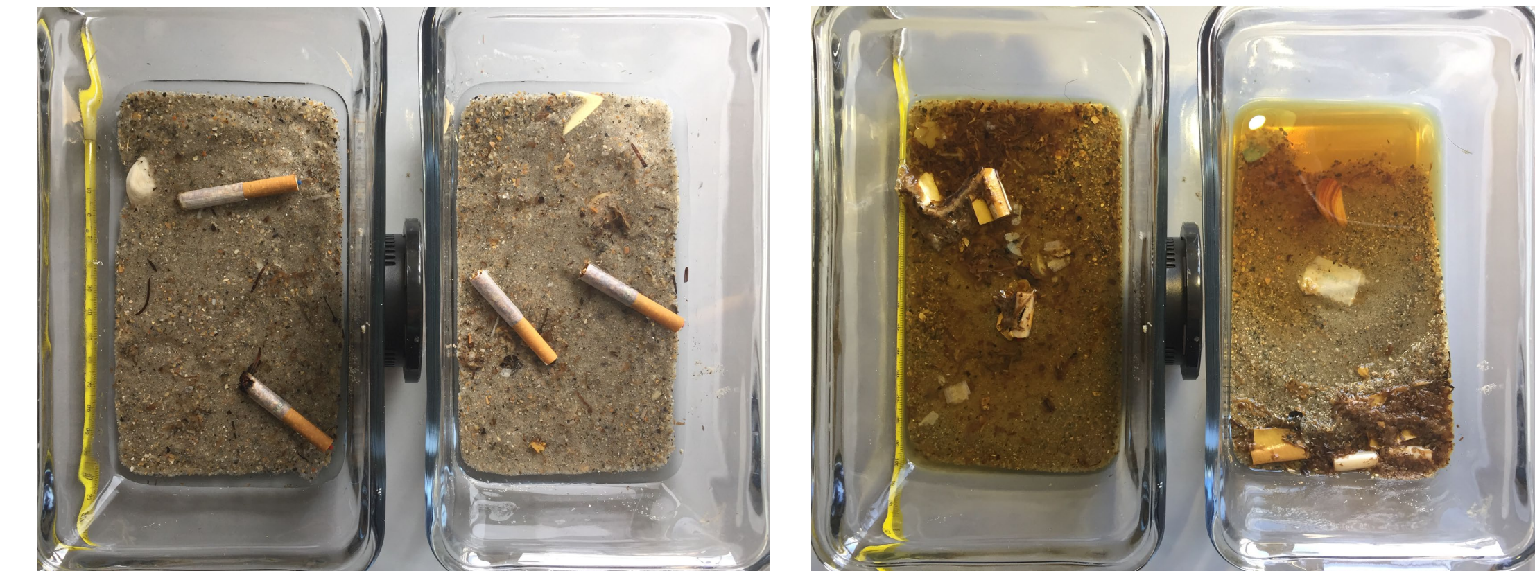
Figures 1 (left) and 2 (right). Pictures of the cigarette butts from Trial 2 on Day 1 (set up) and Day 2, respectively. On Day 2, all four cigarette butts had degraded to filter-only and the water was an obvious copper-brown color.
