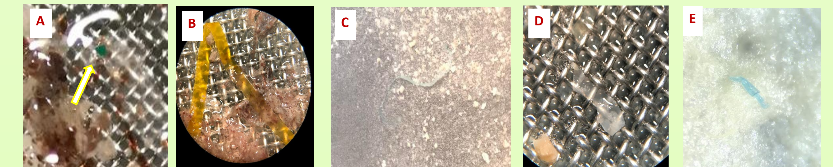
Figure 12: Photographs of possible microplastics collected from the digestive tracts of wild-caught sea bass A) green particle, 63 µm filter, 3x magnification. B) yellow strand, 1 mm filter, 1x magnification. C) light blue fiber, 5 µm filter, 4x magnification. D) transparent film, 1 mm filter, 1x magnification, E) fragment.
